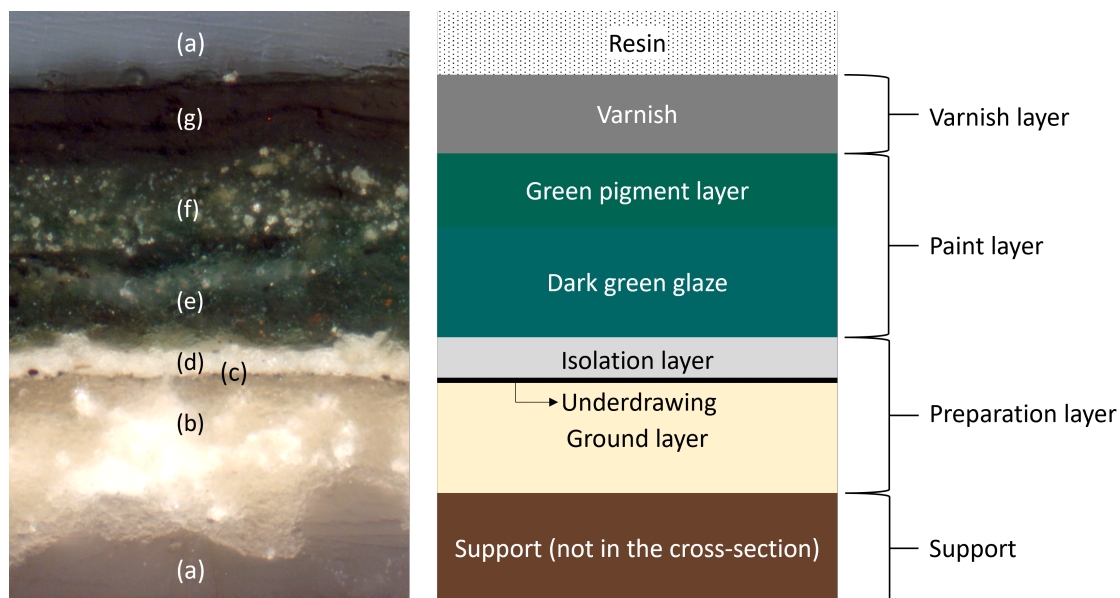
Figure 1.1: Example of layering taken from cross-section C17-085 (more information about this sample in Figure 8.6, section 8.2). The support is not present in this cross-section, but is supposed to lay underneath the ground layer. (a) Resin embedding the cross-section. (b) White ground layer. (c) Bone-black underdrawing. (d) Lead white isolation layer. (e) Dark-green glaze containing copper resinate. (f) Pigment layer containing malachite and lead-tin yellow. (g) Two varnish layers separated by a dirt layer, indicating that varnish has been applied in two different moments.
