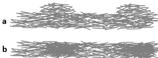
Figure 4.15 – Assumptions about the structure of the mat in the intermediary phase where nanotubes either (a) organize themselves in islets over a nanotube floor or (b) are aggregates in the mat.
