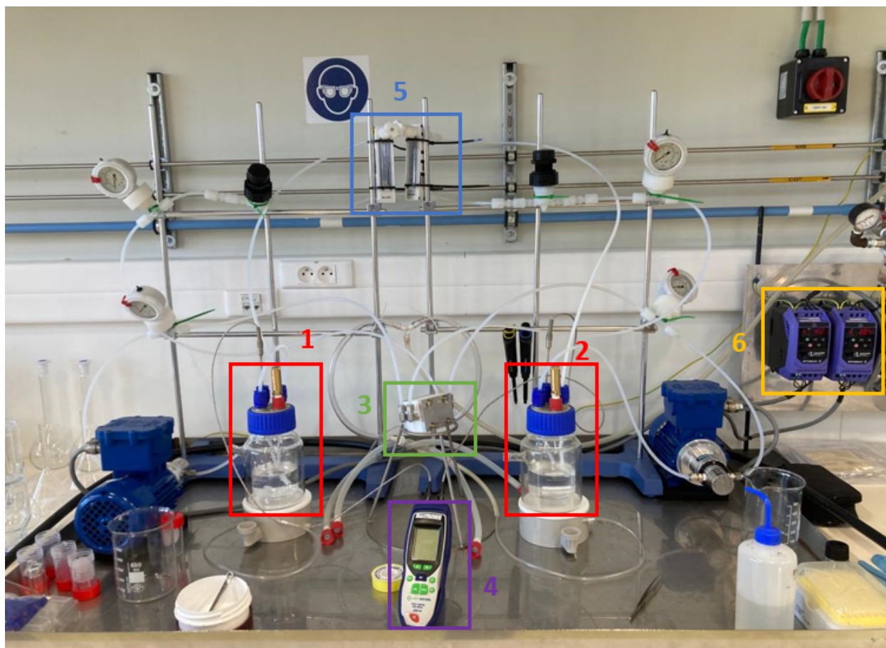
Figure 3.5: Complete set-up used for the membrane extraction experiments. The following part can be identified: (1) the feed solution, (2) the strip solution, (3) the membrane contactor, (4) the digi-sense thermometer, (5) the flow-meters and (6) the frequency drives.
