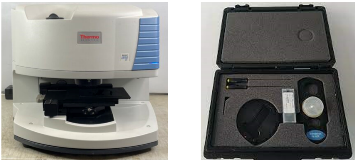
Figure 3.3: Nicolet iN10 Infrared Microscope machine (left) used for the FTIR tests and the plates needed for the FTIR testing (right), obtained from [84].
