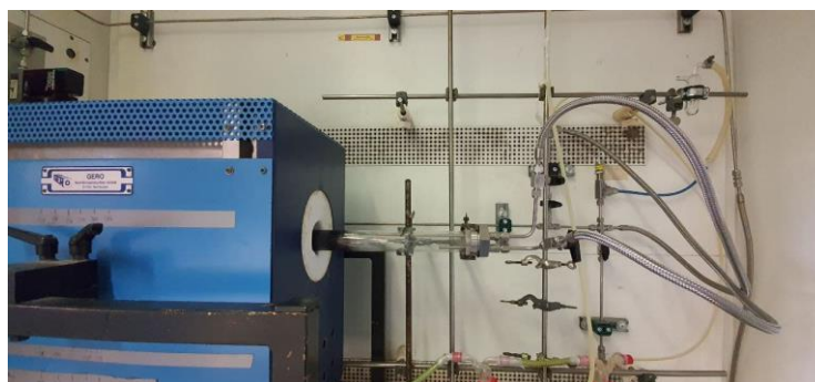
Figure 3-3 Typical setup for Ammonolysis; on the left is the furnace, and the sample is put inside a Schlenk tube, which is sealed and connected to gas inlet and outlet, for constant ammonia flow during the heating cycle.
