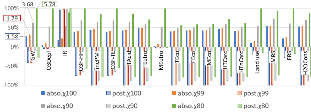
Figure 44 LCIA of absorption and post-treatment with different recoveries \chi - characterisation. abso. \chi 99 refers to the reference case absoA.s0 with ARG and maximum \kappa = 0.561 [mol/kg] and where recovery is \chi = 99\% (i.e. post. \chi 99). All other absorption scenarii with different recovery rates ( \chi = 100, 90 and 80\% ) are operated with ARG and under maximum \kappa = 0.561 [mol/kg]. Absorption accounts for AA recovery whilst crystals and water recovery is credited to post-treatment. Data labels on the bar charts represent global warming emissions in [kgCO 2 -eq]. Abbreviations on the x-axis refer to Table 24.
