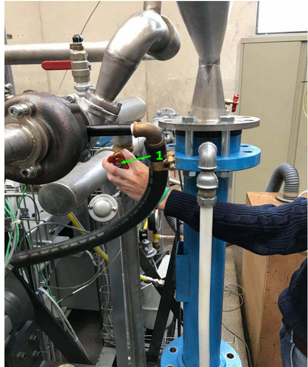
Figure 2.6: Exhaust system: (1) EGR valve.
