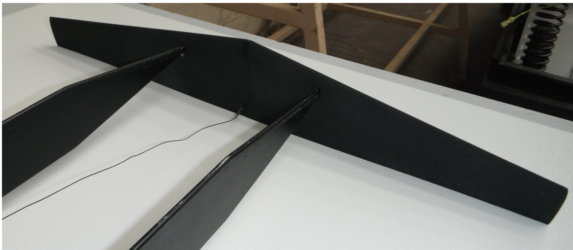
Figure 2.21: Wing painted in black assembled with its support arms
