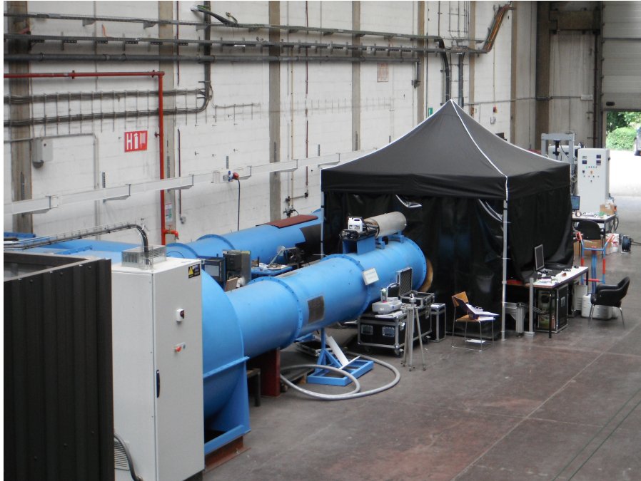
Figure 2.24: An overview of the wind tunnel. The convergent part and the air inlet are in the black tent
