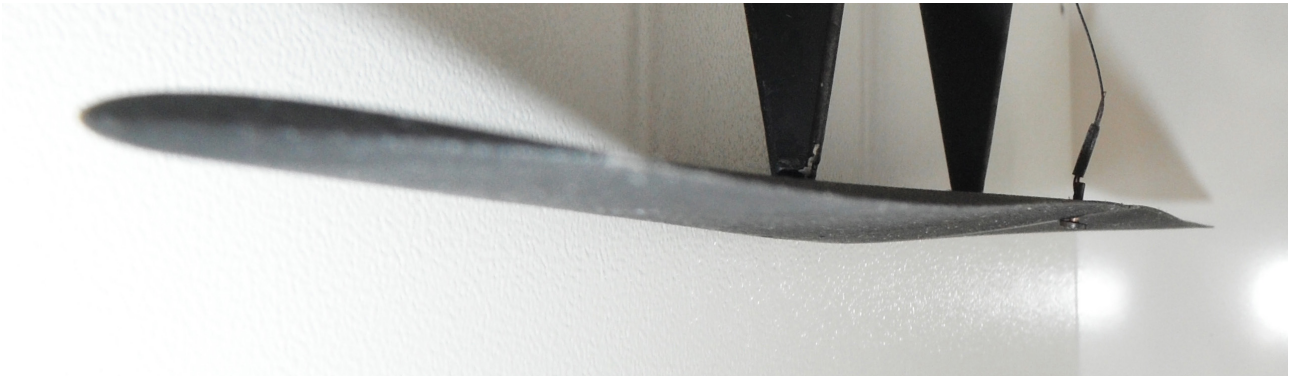
Figure 2.22: Twist visualisation on wing's trailing edge
