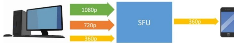
Figure 2.7: Principle of simulcast. [1]
