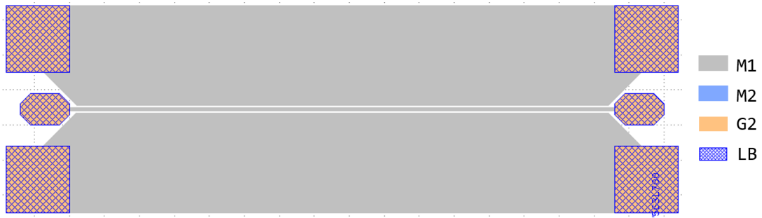
Figure 5.5: Layout of a CPW at M1 line for TV0.
