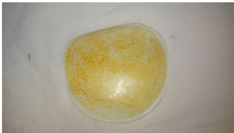
FIGURE 4.11: SILM, [OMIm][NTf 2 ] immobilised in a PAN membrane, after 60 °C with MEOH.
