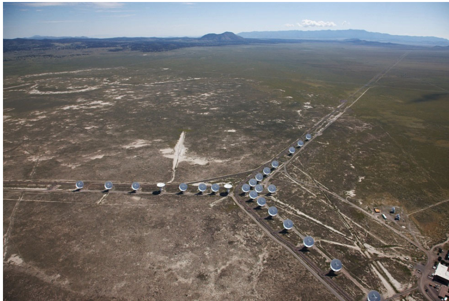
Figure 1.2: Very Large Array telescope in New Mexico. The array is composed of 28 antenna which can be moved on a three-arms star of 20km each[5]
