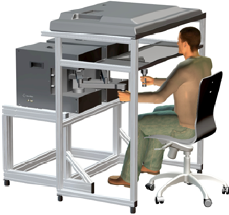
Figure 2.2: Representation of a KINARM End-Point Lab Robot [21]
