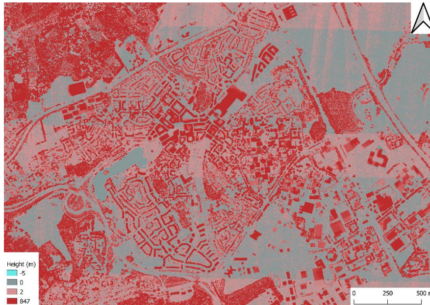
Figure 2. Height dataset (DHM) derived from LIDAR
