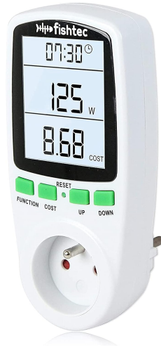
Figure 6.10: wattmeter used for our measurements
