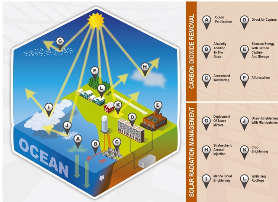
Figure 1: Overview of proposed geoengineering techniques. Carbon Dioxide Removal methods: (A) ocean fertilisation through nutrient input resulting in an increase in ocean productivity and the transport of a fraction of the resulting biogenic carbon downward; (B) alkalinity addition to the ocean from solid minerals enhancing atmospheric \text{CO}_2 dissolution in the ocean; (C) increasing weathering rate of silicate minerals and transport of the dissolved carbonate minerals produced to the ocean; (D) chemical capture of atmospheric \text{CO}_2 and its storage underground or in the ocean; (E) capture of the \text{CO}_2 emitted during biomass combustion in an electric power plant and its storage underground or in the ocean; and (F) \text{CO}_2 storage by land biomass through afforestation and reforestation. Solar Radiation Management methods: (G) installation of reflectors to reflect sun radiation; (H) injection of aerosols in the atmosphere; (I) enhancing marine clouds reflection through seeding; (J) production of microbubbles at the surface of the ocean to make it more reflective; (K) growing more reflective crops; and (L) whitening of roofs and buildings (Boucher et al., 2013).
