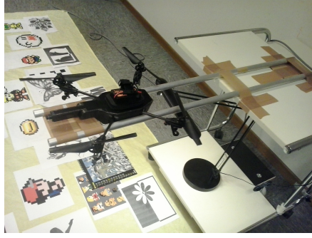
Figure 5.1: Description of the experiment for measuring the visual pose estimation for pure x-y translations
