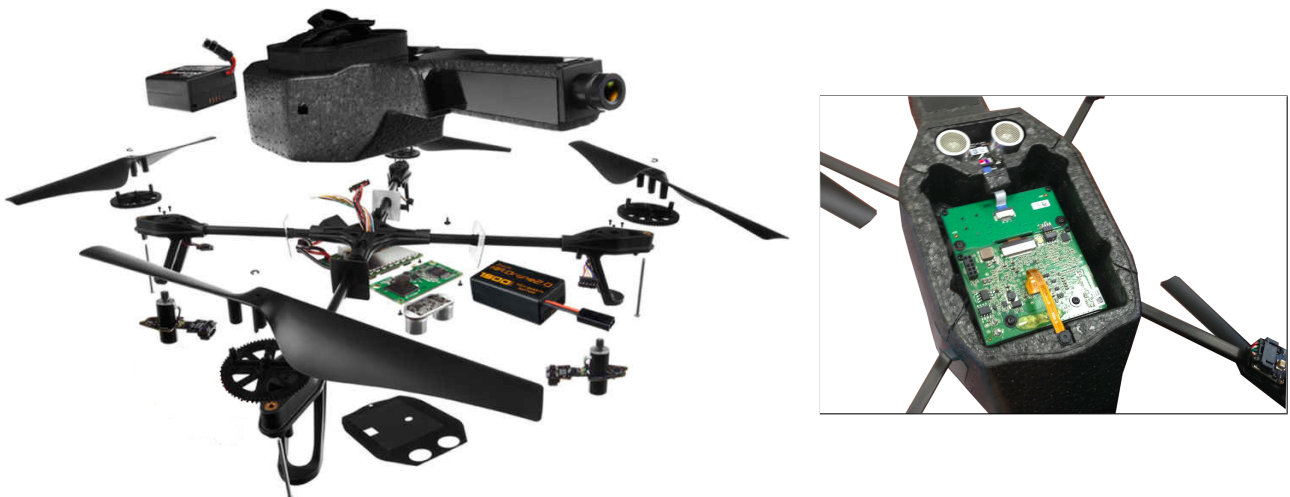
Figure 3.2: Exploded view and inside view of the Parrot AR.Drone 2.0 [147]
