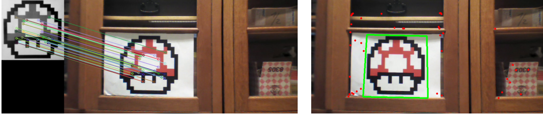
Figure 4.14: Target detection and removing the target keypoints within the green box from the image pipeline
