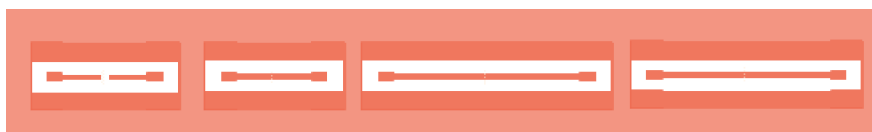
Figure 4.7: Zoom on clock-wised rotated Back-to-back GCPW structures for the mTRL calibration from the mask. From left to right: Reflect (open circuit), Thru, Line 1 and Line 2
