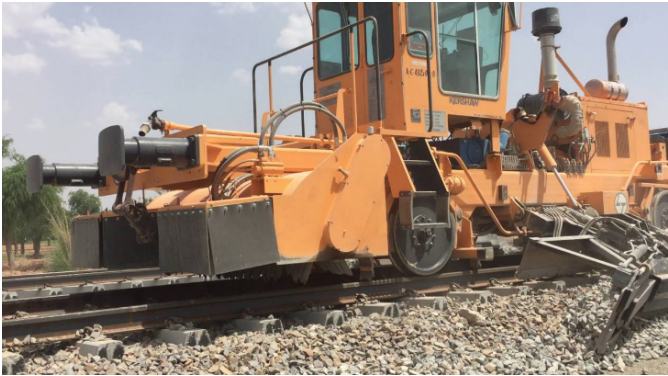
Figure 1.12 – Ballast regulator machine [21]
