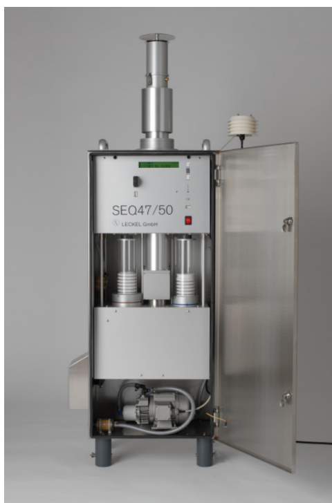
Figure 1.13: The Sequential Sampler SEQ47/50 from Leckel, used in Belgium. Source: http://www.leckel.de/index.php?option=com_content&task=view&id=24&Itemid=68&lang=en .
