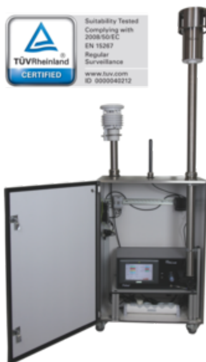
Figure 1.12: The Fidas 200S developed by Palas, Germany, used in Flanders. Source: https://www.palas.de/en/product/fidas200s .
