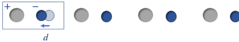
Figure 2.7: Dimerization of the 1D idealized chain which can be induced by a Peierls distortion for instance. The anions are shifted by a distance d to the left.
