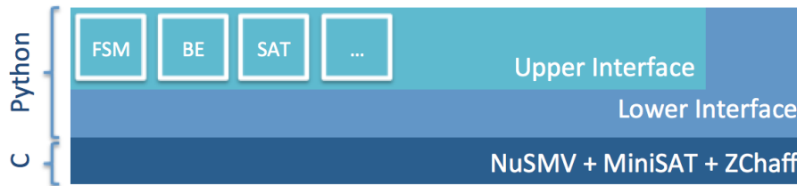
Figure 3.1: Architecture of PyNuSMV with SAT-BMC (Adapted from [10]).
