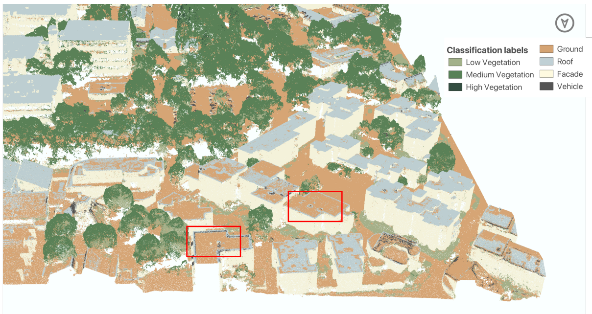
Figure 19. ALL_FEAT classified point cloud showing roof and ground inconsistencies (marked in red).
