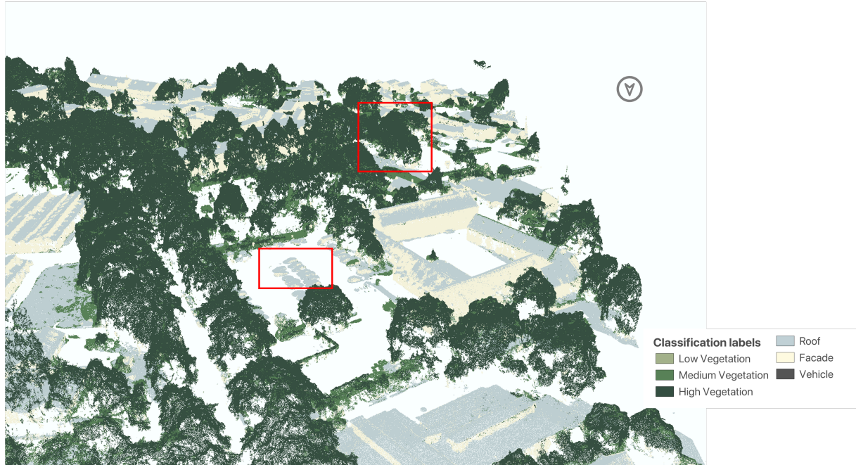
Figure 22. NO_GROUND classification showing vegetation and vehicle inconsistencies (marked in red).
