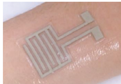
Figure A.4: IDE sensing skin hydration level by change of impedance due to increased dielectric constant [20]
