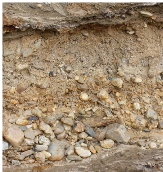
Figure 4.13 MHZ quarry wall 2: fining upward sequence from very coarse gravel to very fine gravel and very coarse sand in unit 3.
