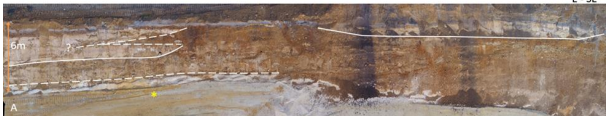
Figure 4.10 Visible units on wall 2 in MHZ quarry mostly large clay plug except one small gravel layer (top). Dashed lines indicate uncertain unit's limits. The yellow marker indicates the position of the profile described in Figure 4.11. Left half of the outcrop is on top, the right side at the bottom.
