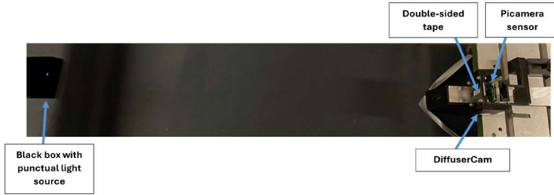
Figure 3.2: Physical installation of the DiffuserCam
