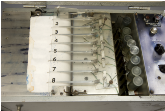
(a) Pen recorder from 1958 for 8 EEG channels [39]
