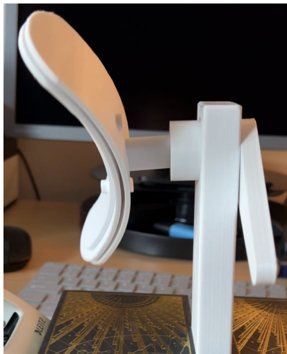
Figure C.1: First method: winding between two curved plates
