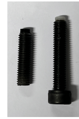
Figure 6.8: Radial (left) and axial (right) soft-tip screws.
