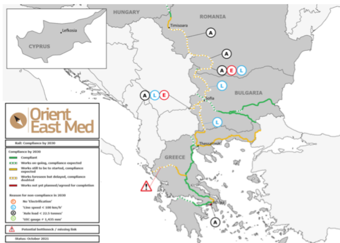
Figure 12: Overview of Rail compliance by 2030 – OEM South
