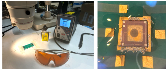
Figure 4.31: Welcome workshop set up for air leakage corrections.
