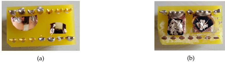
Figure 2.11: Pictures of the two different ways used to mount the samples on a chip: a) or b) by the top or the sample.
