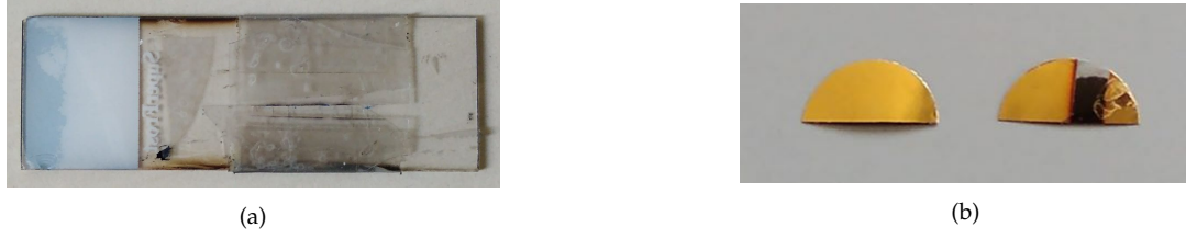
Figure 2.10: Pictures of a) the mask used to etch the samples and b) half an electrodeposited sample before (left) and after etching (right).
