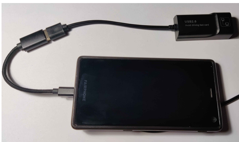
Figure 2.1: Photo representing the micro-USB to Ethernet connection setup using two adapters.
