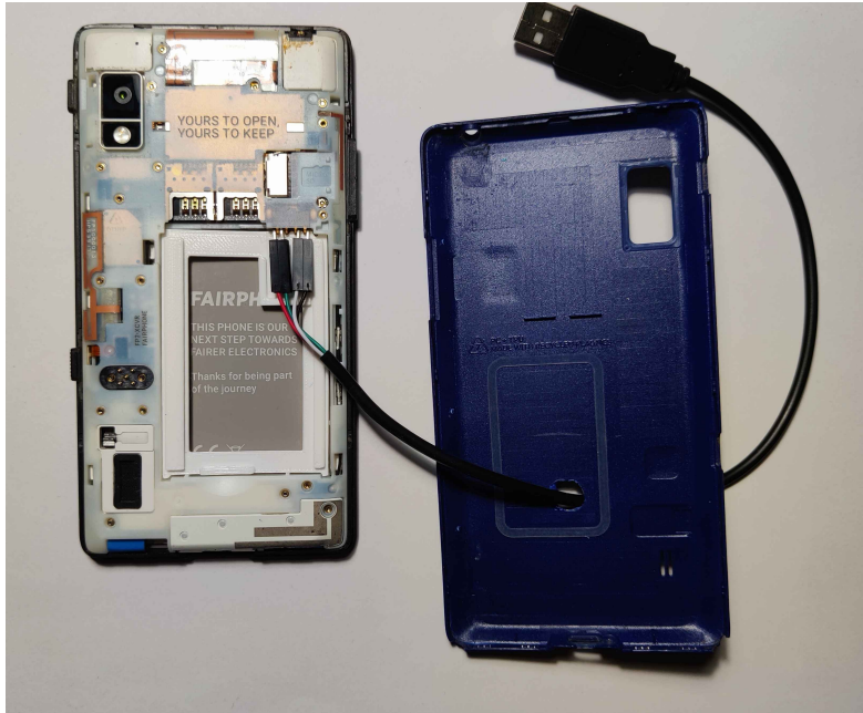
Figure 2.2: Photo representing the power supply adjustments made on the Fairphone 2.
