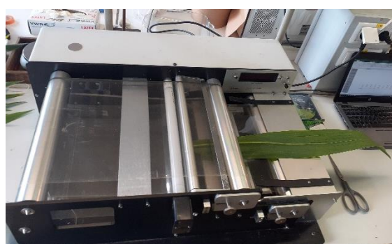
Figure 20 : Scanneur LI-3100c Area Meter (LI-COR)
