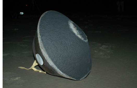
Fig. 1.7: Sample return capsule from NASA's Stardust mission. Picture from NASA 4 taken after landing in Utah [14].
