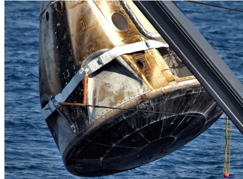
(b) SpaceX Dragon spacecraft and its degraded PICA-X TPS after splashdown. Picture taken by C. Hudson.
