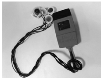
Figure 3.5: Example of an EMG system: the Brainquiry © Wireless system
