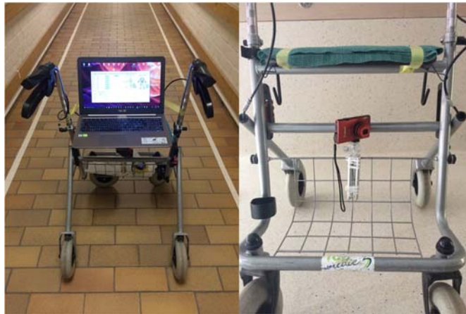
Figure 6.1: IMU and patient's feet camera tracking system
