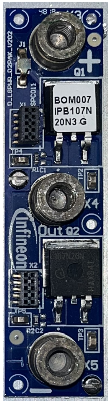
(a) Half-bridge with two IPB107N20N3 G transistors
