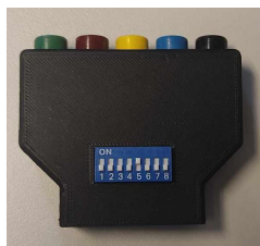
Figure 6.5: Housing used in the experiments to connect the cables of the potentiostat to the contacts of the electrode
