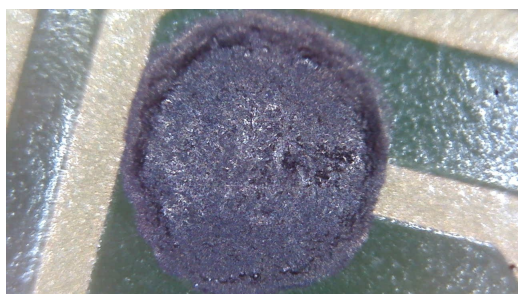
Figure 6.13: Picture of the WE before the EPD process at 5V
