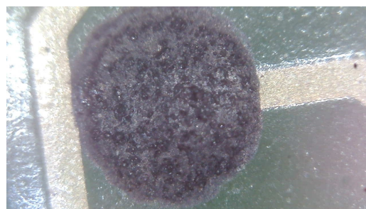
Figure 6.14: Picture of the WE after the EPD process at 5V
