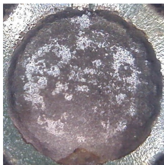
Figure 6.17: Picture of the CE after the EPD at 27V and 5V
