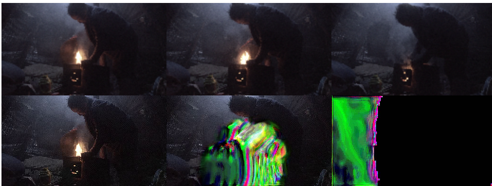
Figure 4.14: Occurrence of an instability in the output of BasicVSR with as input a video composed of 369 downsampled 5 frames to a size of 174 \times 98 . The upper line is composed of some input frames ( 1^{th} , 19^{th} , 61^{th} ) that have been stretched to have the same visual dimensions as the super-resolved images below. Zoom-in for a better view
