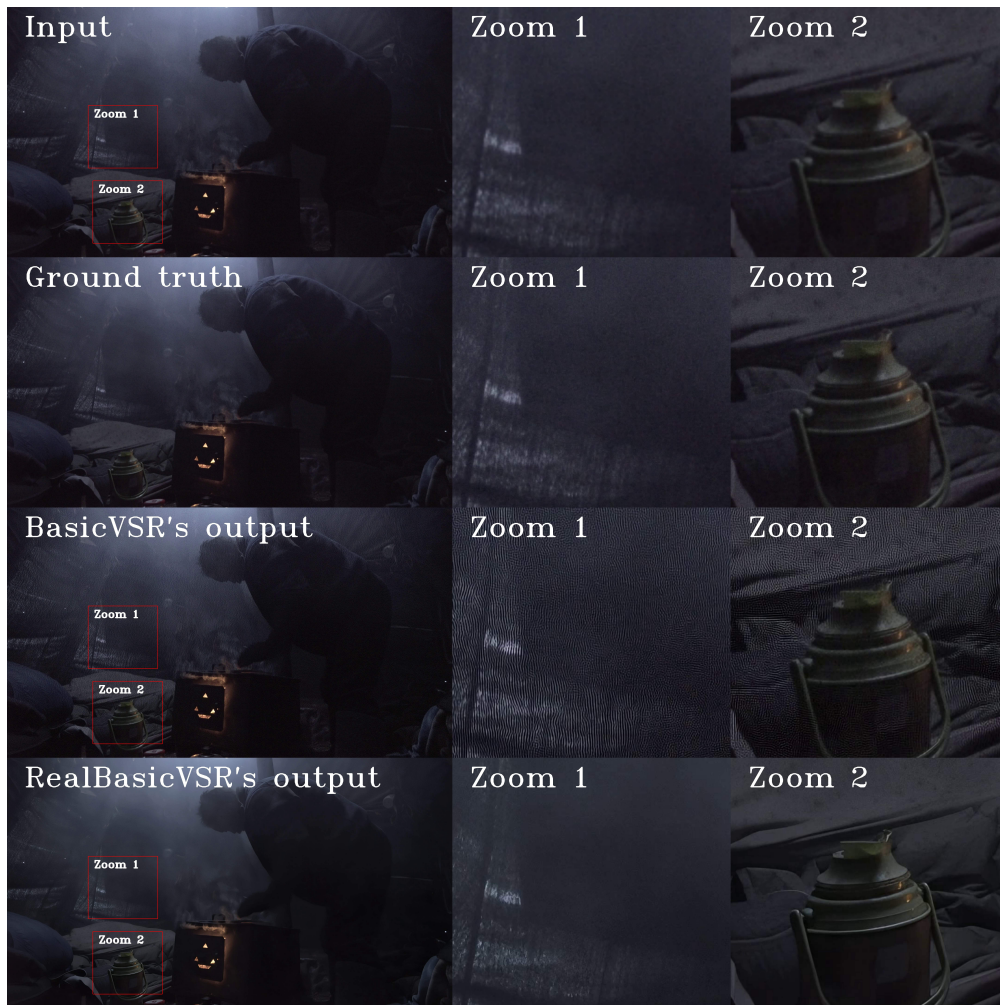
Figure 4.29: Comparison between the result obtained by RealBasicVSR and BasicVSR on a 369 frames long input video downsampled to 960 \times 540 images with l = 20 . The presented image is the 150 th frame of the sequence. For clarity reasons, the input image has been stretched to have the same visual dimensions as the super-resolved image. Zoom-in for a better view
