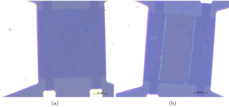
Figure 63: Optical microscope image taken (a) before and (b) after the mechanical cleaning with AFM for a sample of G_3 .
