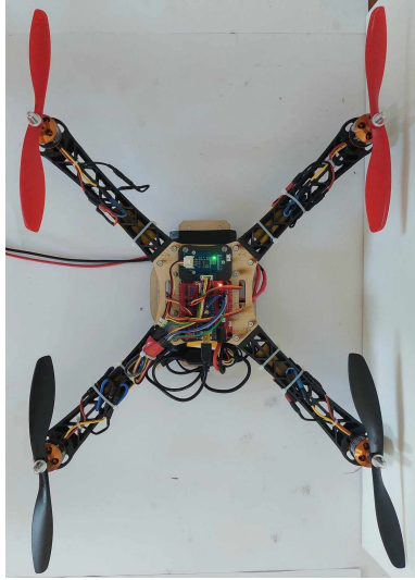
(b) Top view, where the sensing electronics as well as the connection cables are visible
