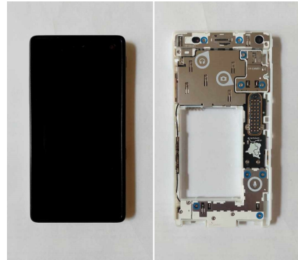
Figure 4.4: Fairphone 2 before and after dismantlement.
