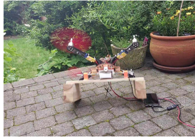
(d) t = 55 [s] due to a step command, the drone is overreacting and losing control.
