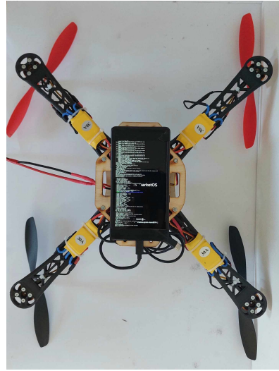
(c) Bottom view, exposing the ESCs as well as the Fairphone 2 (in all its part) powered with postmarketOS.
