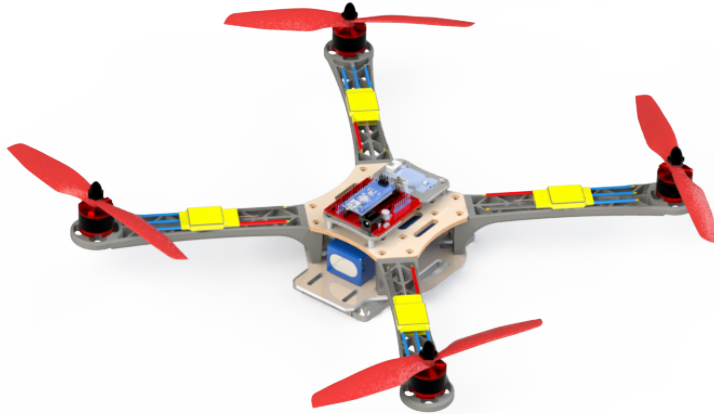
Figure 4.9: 3D developed CAD model of the quadcopter, expressing power electronics (motors, ESCs and battery), the sensing electronics on top of the drone, the FP2 below and the frame (4 arms maintained by 2 wood plate).
