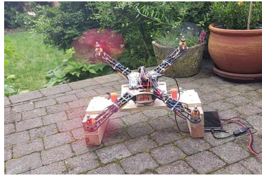
(b) t = 33 [s] the drone is inclined with a positive roll [ \sim 30^\circ ]
