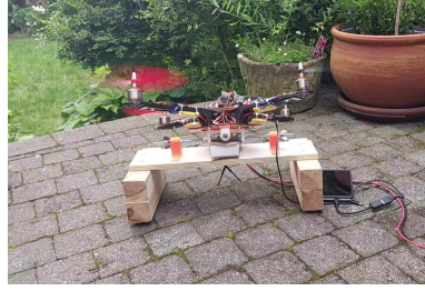
(a) t = 25 [s] the drone is inclined with a negative roll [ \sim 10^\circ ]
