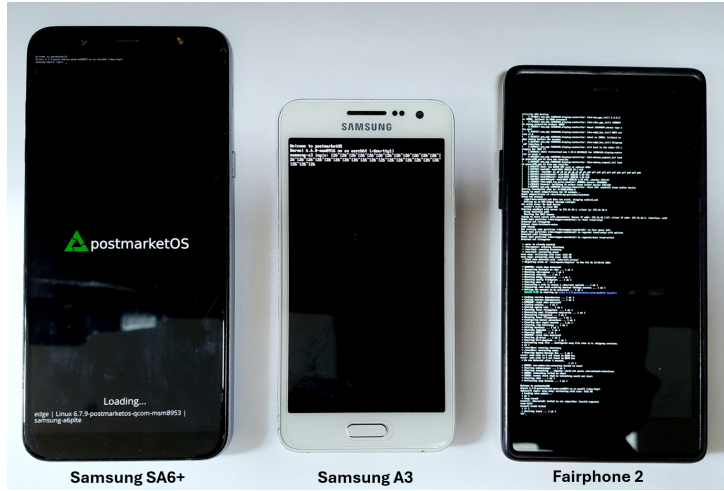
Figure 4.3: Picture of the three selected discarded smartphones with pmOS installed with the minimal graphic interface selected.
