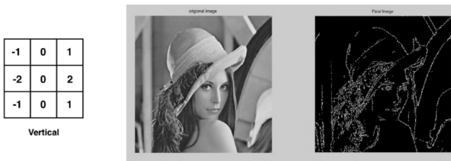
Figure 2.11: Convolution effect on an image [7]
