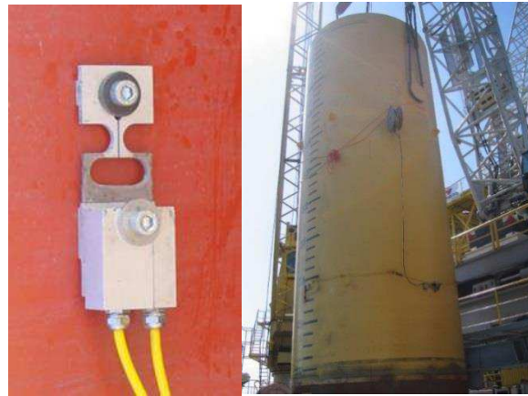
Figure II-8: Strain gauge and accelerometer combined sensor (left), Riffgat monopile (right)
