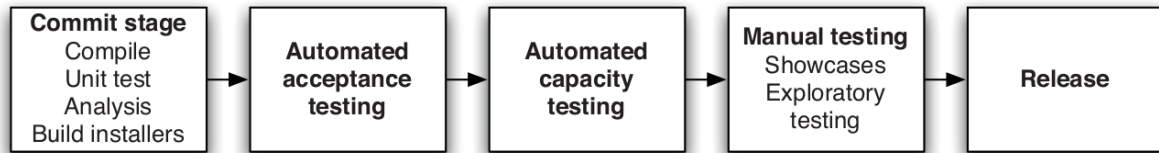
Figure 2.1: Continuous Delivery - Deployment Pipeline
