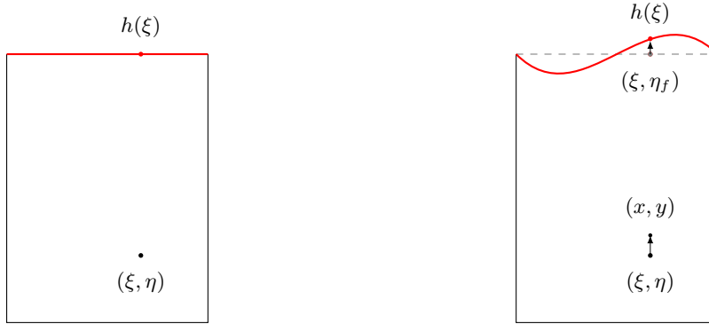
Figure 4.1: Illustration of regularization. The free surface, represented in red, is deformed using the kinematic condition. The inner nodes are moved vertically to satisfy Equation (4.6). Their new position is denoted by (x, y) .
