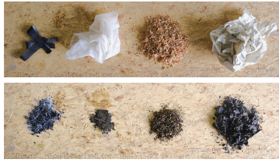
Figure 3.3: Fuels selection from left to right : Rubber tube, LDPE plastic, Wood chips and Paper. The above image shows 30 grams of each fuel untouched. The second image below corresponds to the fuels harvested after combustion.
