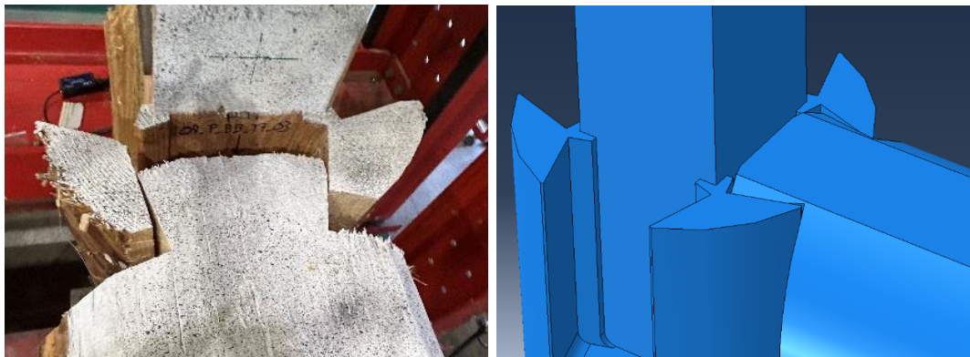
Figure 62: Zoom on the dovetail assembly. Left: experiment in laboratory when the fracture has happened (source: Serena Van Nimwegen). Right: 3D model.
