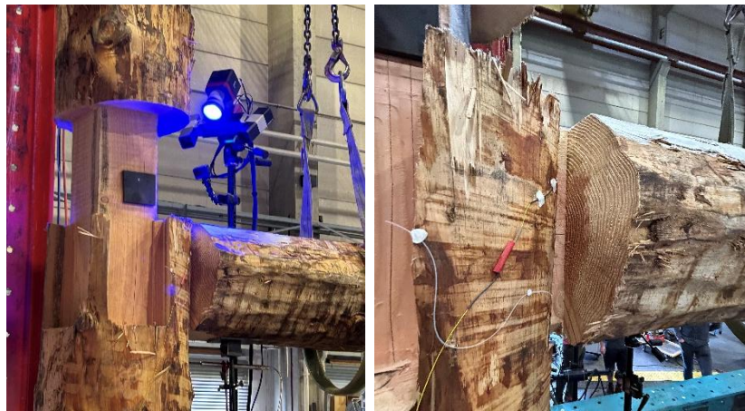
Figure 64: (left) View of the cameras required for the DIC. (right) View of the location of the LVDT's on the column (same on each side of the column).
