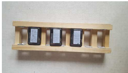
Figure 3.19: Structure to tare the IMUs
