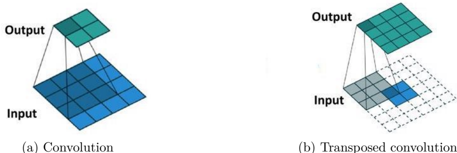
Figure 1.6: Illustration of a convolution of a 3 \times 3 kernel over a 4 \times 4 input and a transposed convolution which is equivalent to a convolution of a 3 \times 3 kernel over a 2 \times 2 input padded (introduction of new pixels around the edges of an image) with a 2 \times 2 border of zeros [14]
