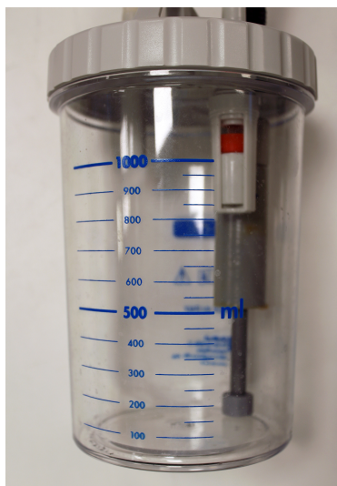
(A) Collection container with the volume graduations and the non-return valve.
