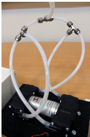
(A) Vacuum pump and its parallel tubing connections.
