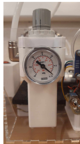
(B) Vacuum regulator, its knob above and its integrated gauge.
