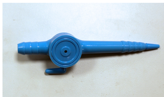
FIGURE 4.1: Vacuum arrest mechanism featuring an upper perforation to prevent air ingress.
