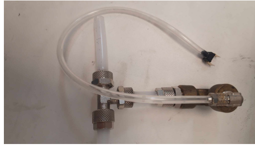
FIGURE 3.18: Series connection in the vacuum circuit. The example is illustrated with the pressure transducer.
