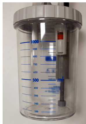
FIGURE 5.12: Collection container level indicators.
