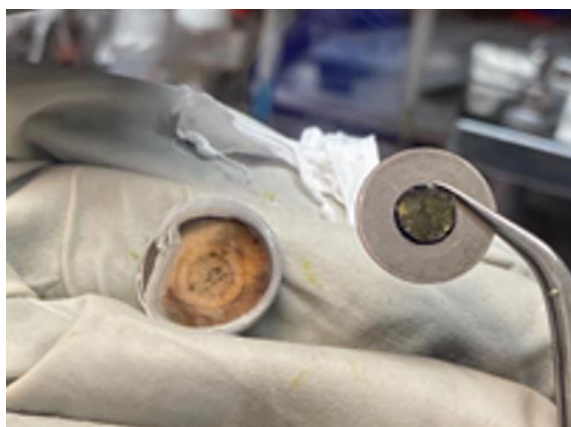
Fig. 20 Solubility issue in cycled \text{Li}_4\text{-}p\text{-DOBDA} at separator (electrode side, left) and the active cathode material at cathode case side (right)
