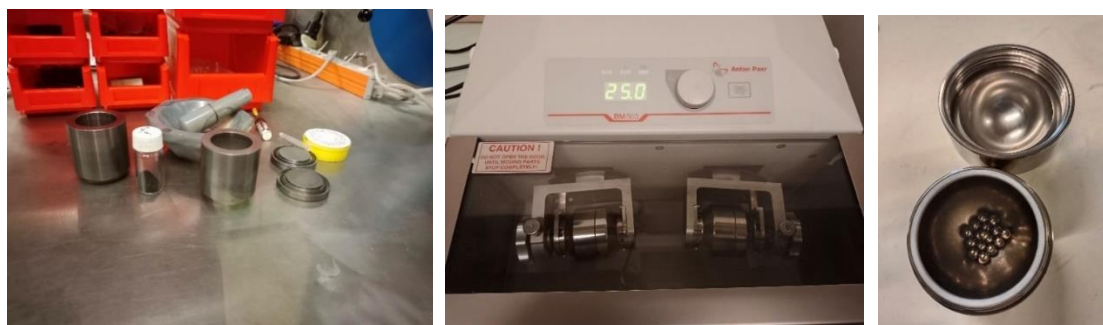
Fig. A4 Stainless steel jars and equipment for Ball Milling (There is equivalent number of balls to make identical weight, only 1 jar is shown with ball)
