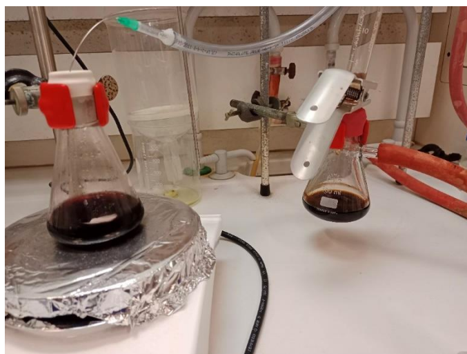
Fig. A9 Observed Colour change during Synthesis using Schlenk Tube Method (left, after long stirring duration) and Ambient Air Synthesis (right after mixing and gets stirred)
