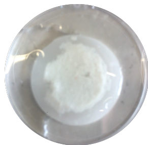
Figure 3.7: Picture of a 3-layered nanopaper before adhesion improvement. A drop of polyelectrolyte was placed over the nanopaper, to form a complex to improve the cohesion of the structure.
